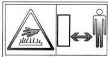
△Notes of the action of the working equipment—Paste it both sides of the dipper.
